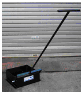
pulling bucket with hinged handle, dimensions: 200 x 300 mm, approx. 1.000 mm long handle other dimensions available upon request
