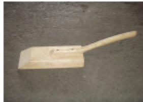
asphalt-float made of hard wood, two pieces
